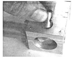
Place the cable rod pin into the shifter.
