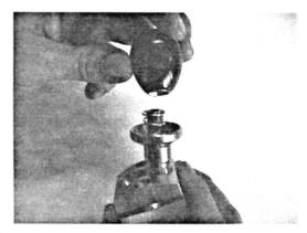
When installing the knob, use low strength loctite. Don't thread all the way down. Make sure first that the shifter can shift clear.
