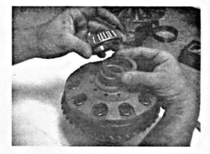
Install your bearings and shims in accordance with your MSM. Note: installation kit not included – bearings, shims, etc.
