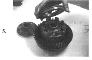
Install locking ring gear with gears facing engagement with locking side gear
