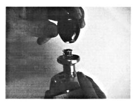
When installing the knob, use high strength loctite. Don't thread all the way down. Make sure first that the shifter can shift clear.
