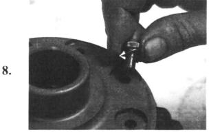
Install the  $\frac{1}{4}$  bolts and spring washers. Apply high strength loctite to bolts.
