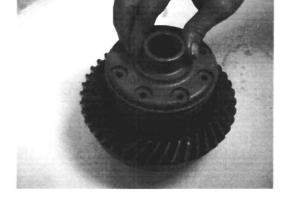
Install small carrier cap – align holes, make sure it slides into locking side gear smoothly.
